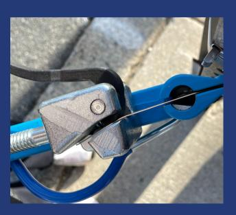
(Wrapping band around pole\bin) (Make sure you insert the band fully into each part of the tool)
